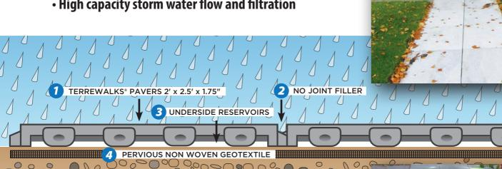
TERREWALKS® directs stormwater to the joints and flows at a rate of 420 cu in/hr.
